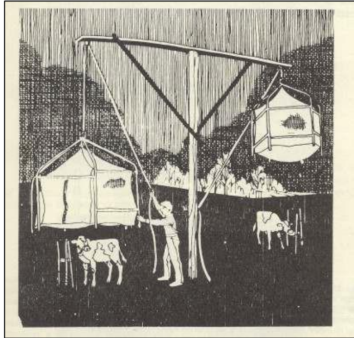
Drop trap for collecting Culicoides attracted to tethered calves
